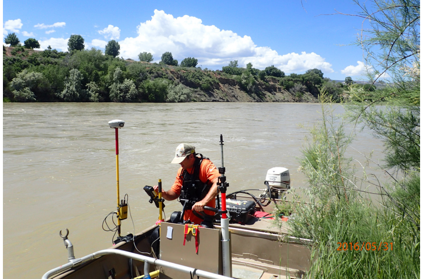
Single beam 5 degree GPS integrated sonar for reliable measurements in turbid waters
